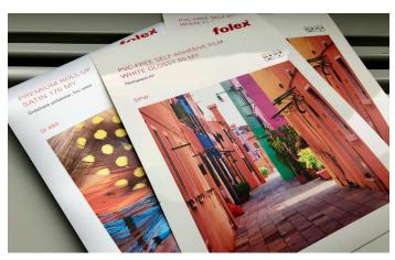
SI 484 is a B1 fire resistant certified film which now includes a new EU fire resistant certificate EN-13501-1, uniquely in the market, the film uses a PET base film, with a reverse side grey layer block out. The film has an attractive, print receptive, satin surface suitable for solvent, latex and UV inks
